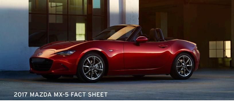
Lighter, smaller, quicker and more nimble than its predecessor, MX-5 has adopted Mazda's full suite of SKYACTIV Technology and KODO-Soul of Motion design. In the process, MX-5 has shed approximately 150 pounds from its predecessor, with a curb weight of 2,332 lbs. when equipped with SKYACTIV-MT six-speed manual transmission (2,381 lbs. with the six-speed automatic transmission).
